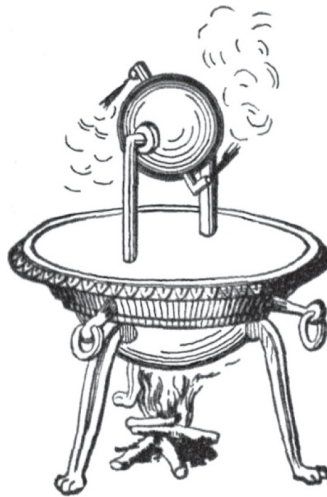
Aéolipile, Héron d'Alexandrie, 1 er siècle ap. J.-C. (image domaine public, source Knight's American Mechanical Dictionary, 1876)
